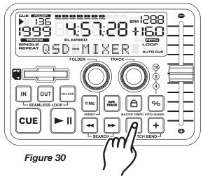
Holding down on the (+) PITCH BEND BUT-TON (29) will provide a speed bump in the playback pitch.
